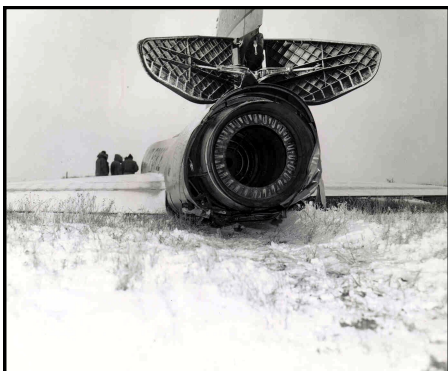
▲ The open doors of the drag parachute compartment above the engine tailpipe prove that Lieutenant Foust deployed the 'chute, as called for by recovery procedures, in his vain attempts to stop his aircraft's flat spin.
