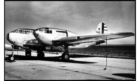
▲ Bell modified the last three pre-production Airacudas into YFM-1As, with tricycle landing gear, revised canopies and nacelles and non-turbo-supercharged engines. Bell's experience with the YFM-1A aided the company in designing the renowned P-39 Airacobra, the world's first production aircraft with retractable tricycle landing gear.
