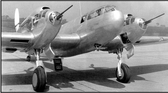
▲ The Airacuda looked a little ungainly on the ground, especially the tailwheel versions. This photo of the prototype XFM-1 shows several interesting design features. Note the cannons and machine guns, the air intake scoops atop each nacelle, the crew entry doors under the fuselage and in each nacelle, and the circular turbo-supercharger exhaust just behind the crewman leaning from the right nacelle with his arm on the canopy sill.
