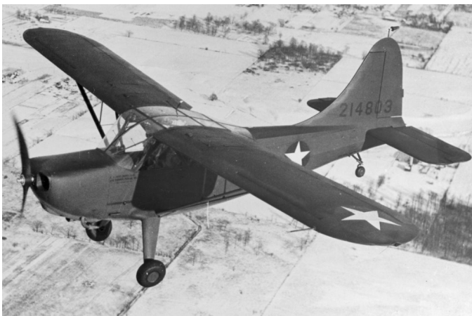
▲ This very nice in-flight view of Stinson L-5 Sentinel serial number 42-14803, the fifth L-5 off the production line, is from the website www.stinsonflyer.com and presumably shows the aircraft during a shakedown flight near the Michigan factory in the winter.
