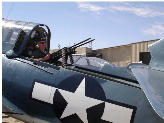
▲ CAF Colonel Ted Short demonstrates the rear gunner position of the Helldiver . One of the more interesting features of the aircraft is the upper rear fuselage between the gunner’s position and the tail, which is retractable in order to provide a clear field of fire for the twin Browning .30-calibre machine guns. Only the gunner’s training prevented him from shooting off the tail—there was no mechanical or electrical interrupter to stop the guns from firing if they were aimed at the tail.
