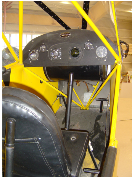
As simple as it gets—stick, rudder pedals, throttle and six flight instruments in the cockpit of the Museum's J-3 Cub.
